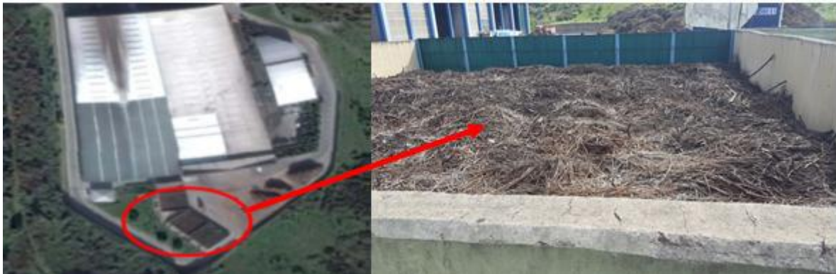
Figure 3. Open bed biofilter unit where the study was carried out (Çelikten, 2018).
