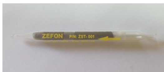
Figure 4. Glass tube used in volatile organic compound sampling (Çelikten, 2018).
