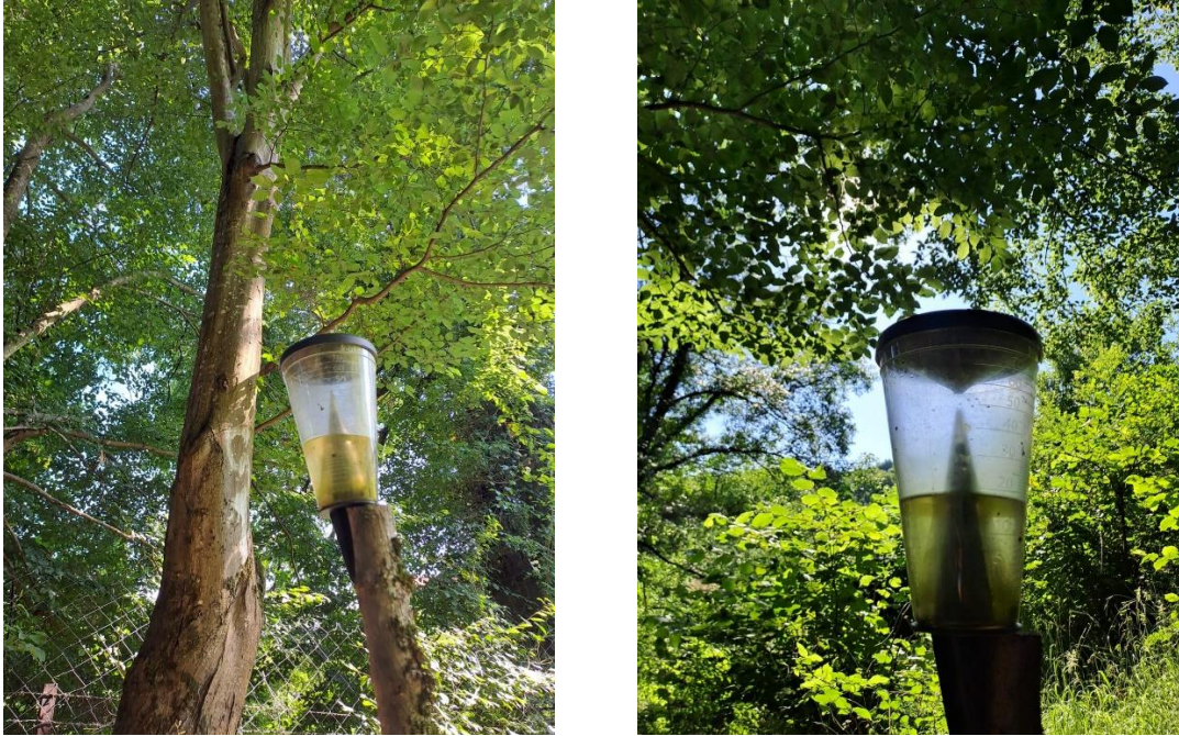
Figure 1. Pluviometers used to measure throughfall
