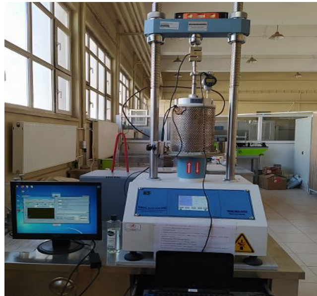
Figure 6. Unconfined compression test apparatus
