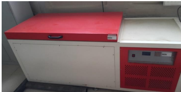
Figure 4. Programmable freeze-thaw cabinet
